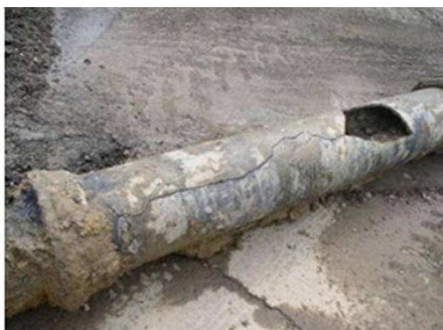
Figure 4. Breakage of a cast iron pipe as a result of hydraulic hammering
