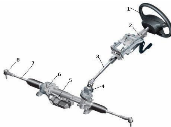
Figure 2. Rack and pinion steering structure:
