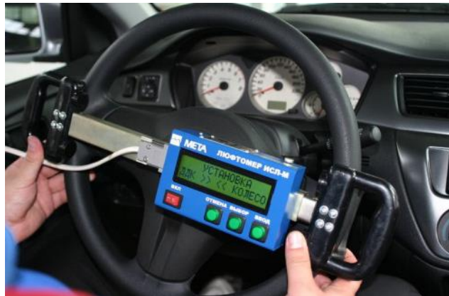
Figure 3. Determining the steering wheel luffi using the lupmer
