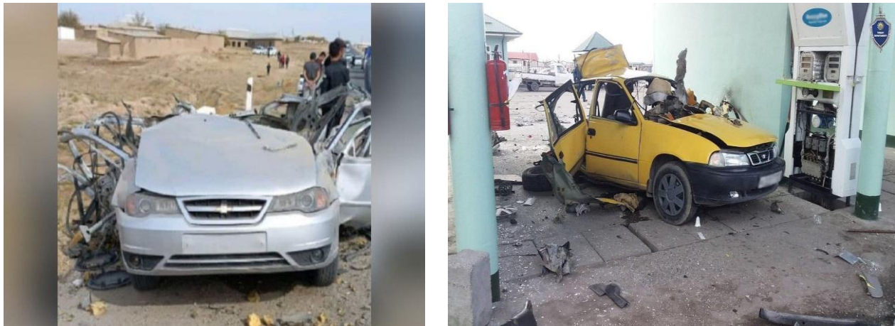
Figure 1. Exploding of gas cylinders due to over pressurization of gas cylinders and neglect of technical operational requirements.
